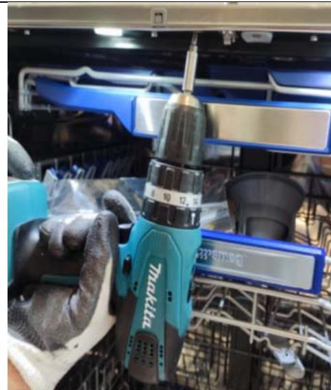
6. Remove the lock fixing screws
