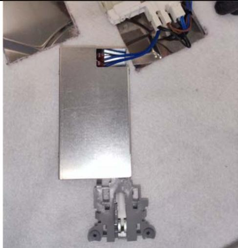
12.13 Connect the wiring to the clamps of the new lock, code **69613C416**
